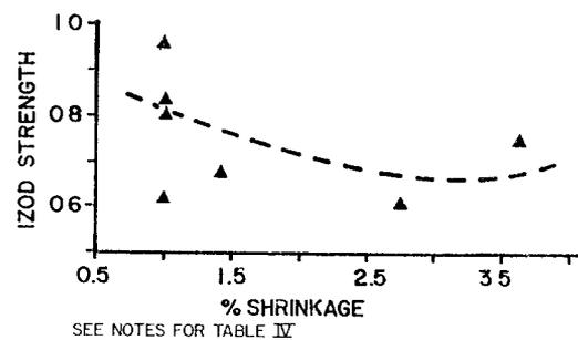
without weldline. In samples containing a weldline high orientation yields low strength. (See Graph VIII.)
