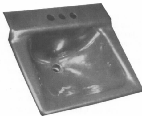
Figure 2. An example of a structural foam part with a smooth, glossy surface.
